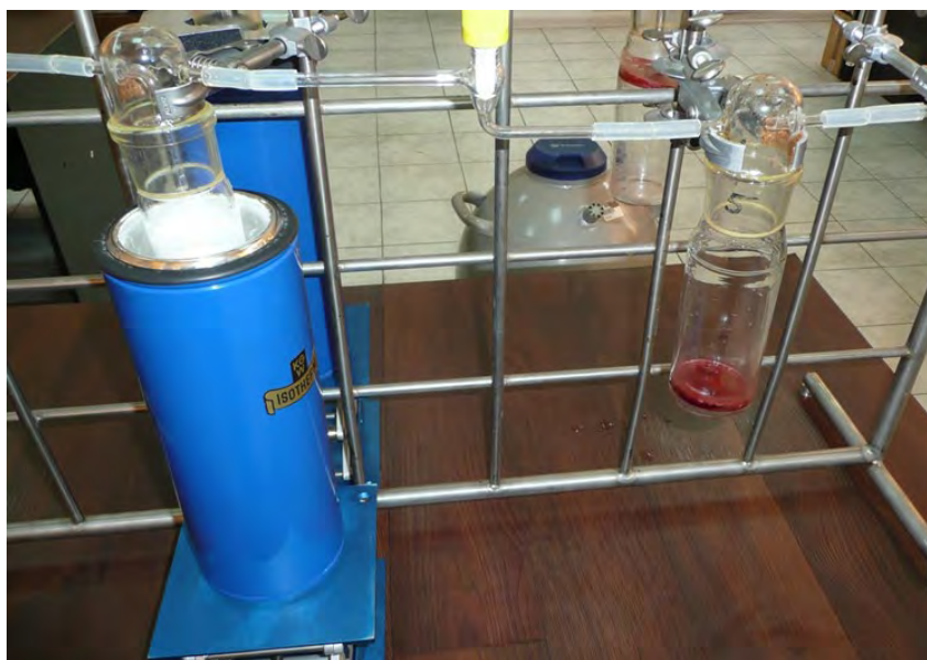
Figure 1: Lyophilization installation for purification of water samples for tritium analysis.
